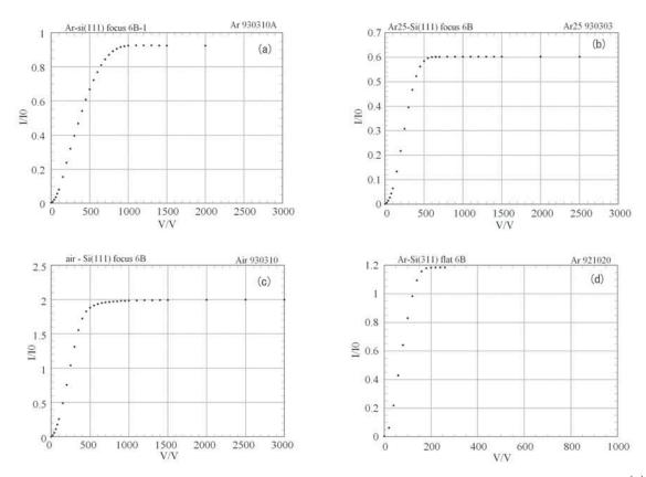
Fig. 2. Saturation curves of an ionization chamber. Incoming flux is similar among (a) to (c) but lower (d). When heavier gas is used, apparent saturation voltage increases except the case of air.
