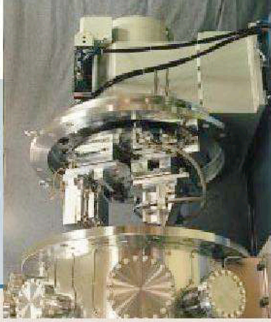
Crystal adjustment mechanics of HLD-1 monochromator.
